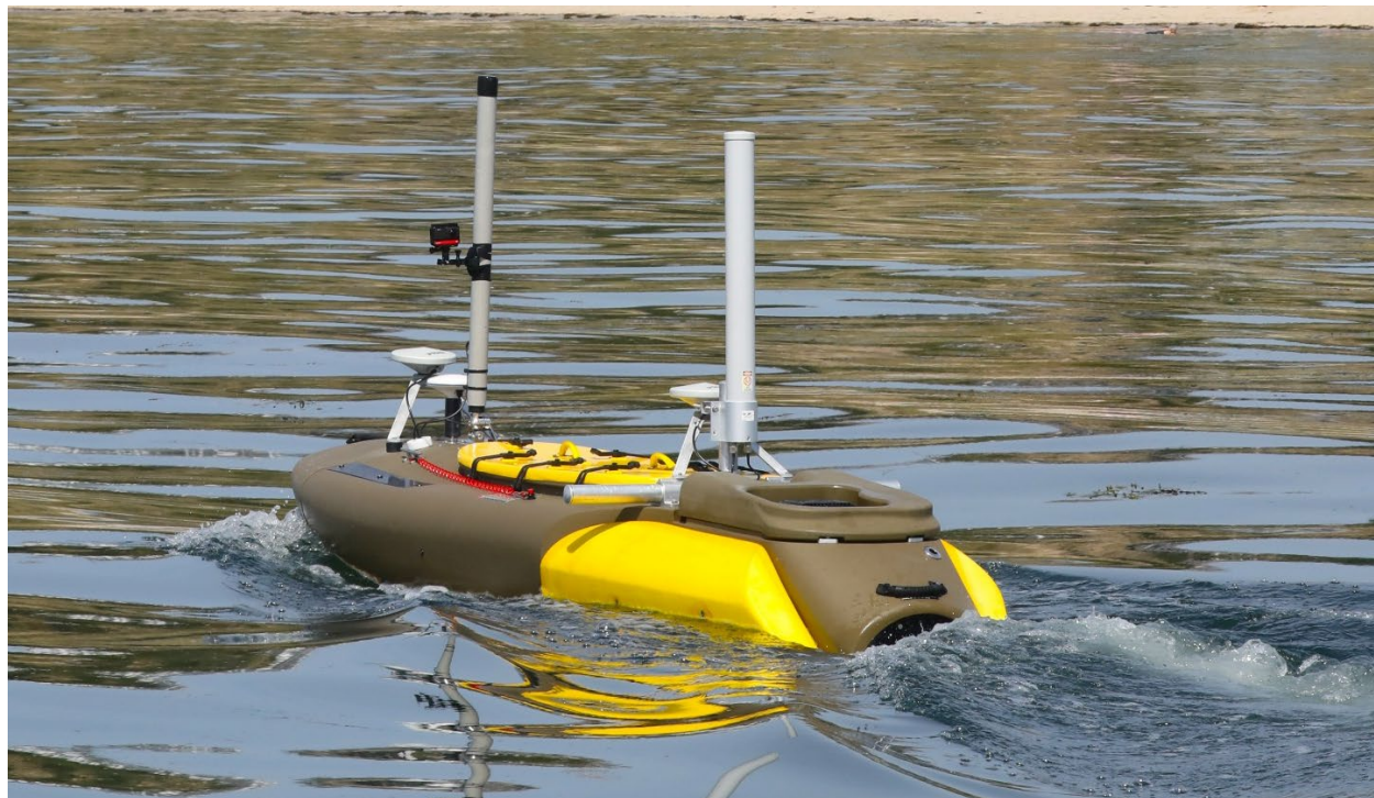
Figure A.3. ASV Jetyak, a hybrid unmanned vessel supporting remote and autonomous operations with real-time monitoring and sensor integration.
