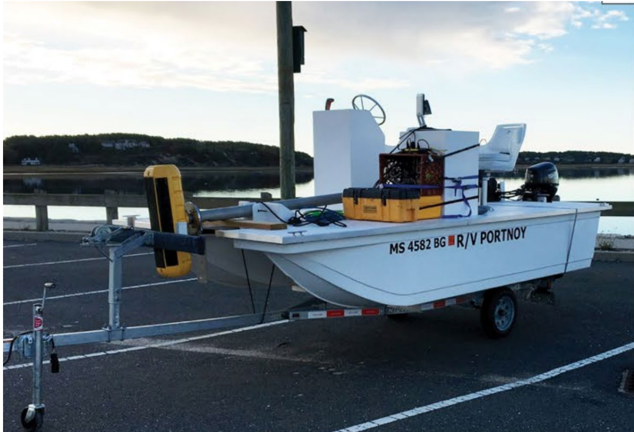
Figure A.2. R/V Portnoy is an ultra-shallow draft pontoon survey vessel, custom-built for high-resolution data collection in low-energy embayments and wetlands. It is shown here equipped with an EdgeTech 6205 sonar system mounted on a bow pole.
