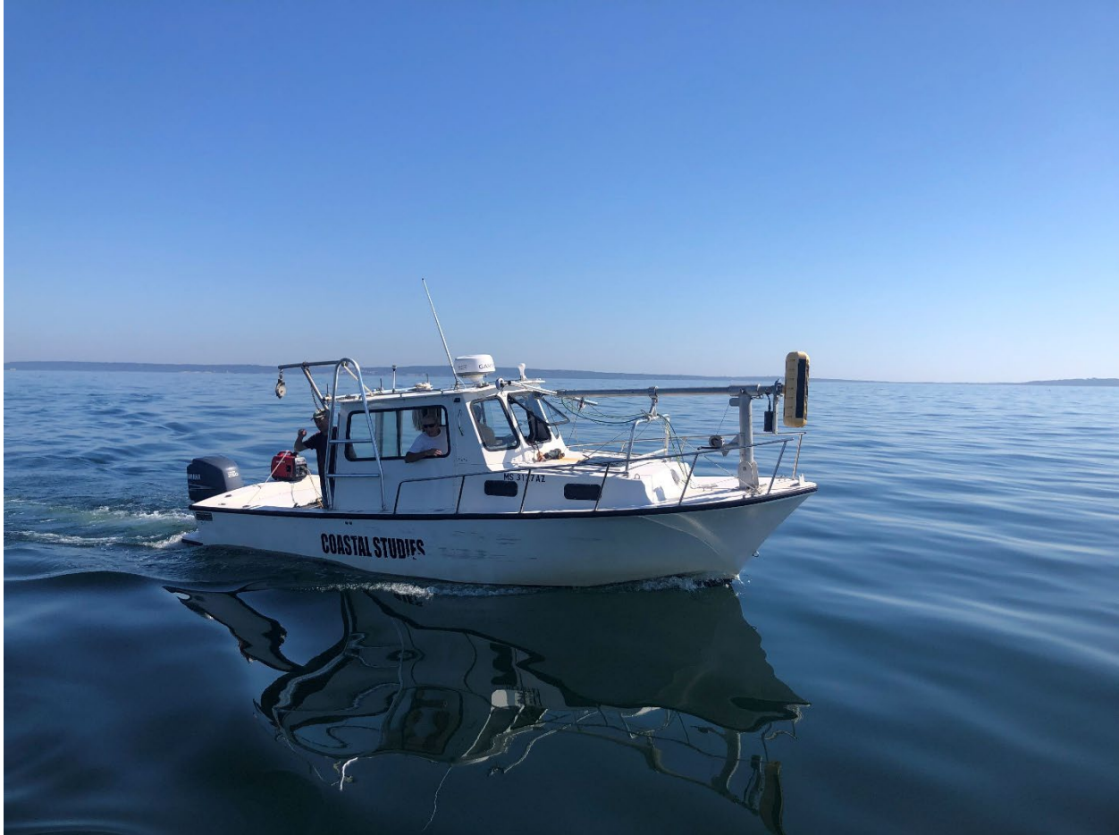
Figure A.1. R/V Marindin survey vessel equipped for shallow and nearshore bathymetric operations, showing retractable bow-mounted Edgetech 6205 system.
